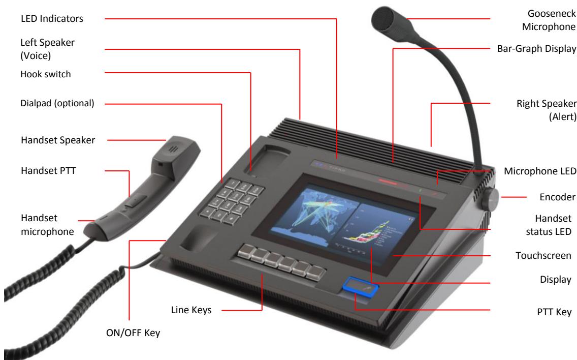
Figure B.1 Operator Interface of BeFREE07
