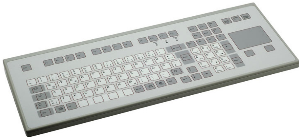
Figure 2. Standard Layout with Integrated Touchpad (K547)
