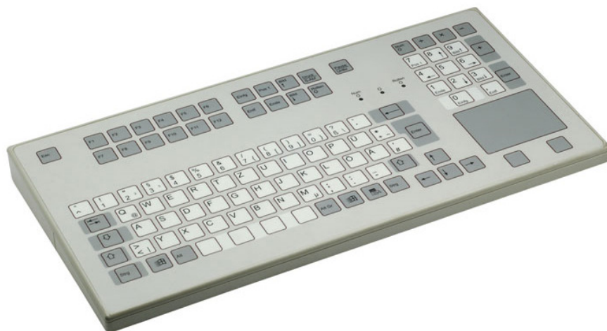
Figure 3. Compact Layout with Integrated Touchpad (K548)
